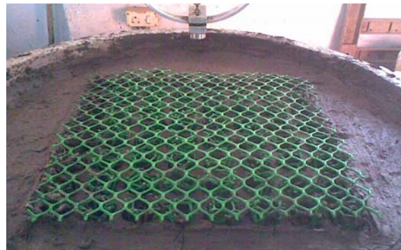
Figure 7. Tying of top surface the of circular geogrid cage
