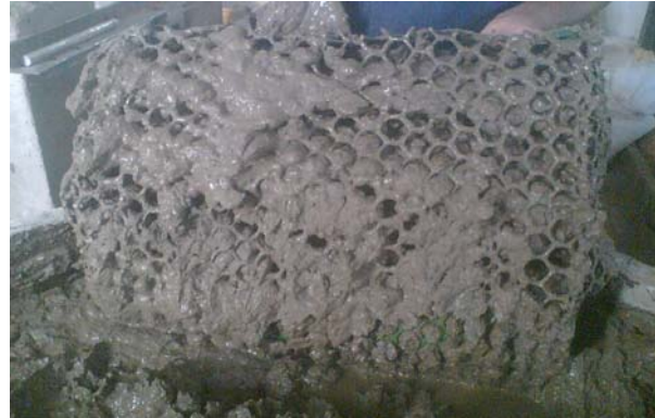
Figure 5. View of removed geogrid after testing
