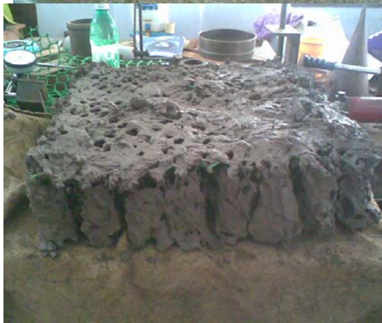
Figure 14. Installation of wick drains
