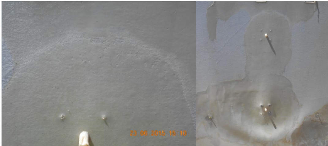
Figure 5. Injection profile around the injector (left) and interface between two injection spots (right)
