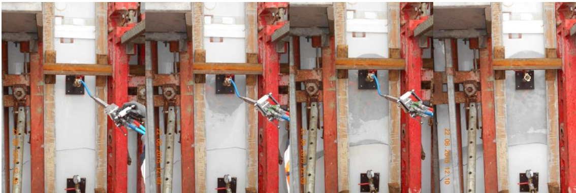
Figure 4. Radial displacement during injection of Resin \alpha from the second point of injection and contact with the first injection
