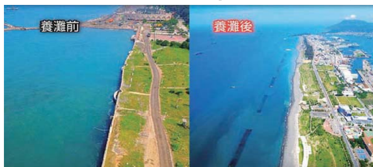
Fig. 19: Offshore submerged breakwaters with nourishment schemes were used for Kaohsiung harbor beach protection project (Kao, 2013).
