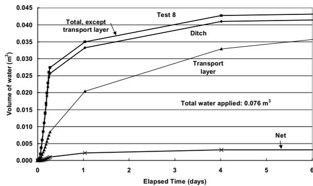
Figure 7. Outflow measured from Test 8.
