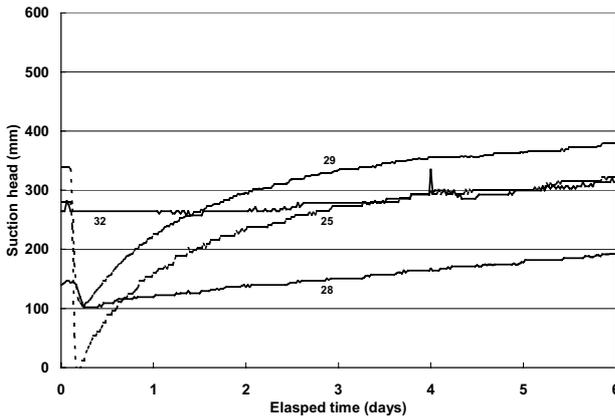
Figure 12. Suction heads in base, 13 mm above the GCBD in Test 9.
