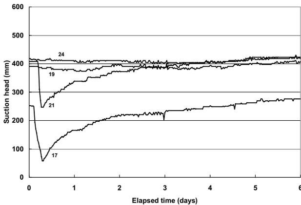
Figure 6. Suction heads in the subgrade, 25 mm below the GCBD for Test 8. Water was applied for 6 hours, for the first 0.25 days shown.
