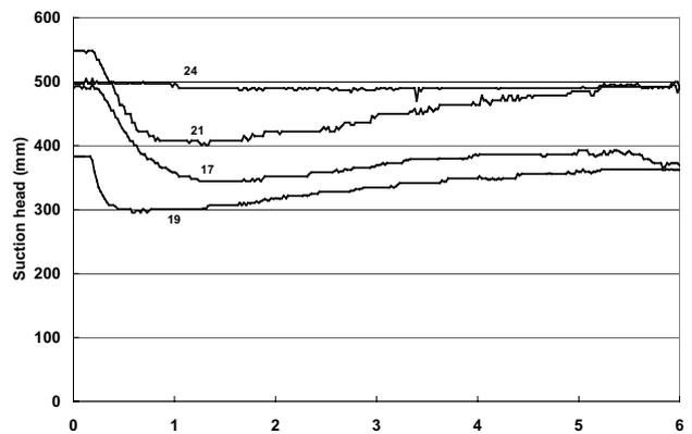
Figure 10. Suction heads in the subgrade, 25 mm below the separator in the control section for Test 3.
