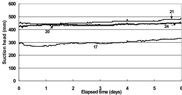
Figure 11. Suction heads in subgrade, 25 mm below the GCBD in Test 9.
