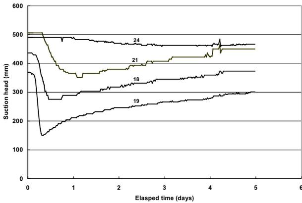
Figure 5. Suction heads in the subgrade, 25 mm below the separator in the control section for Test 4 (control section). Tensiometer 17 did not function properly for this test. Water was applied for 6 hours, for the first 0.25 days shown.
