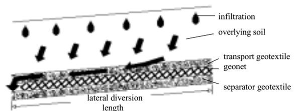
Figure 2. Geocomposite Capillary Barrier Drain (GCBD) with overlying soil.
