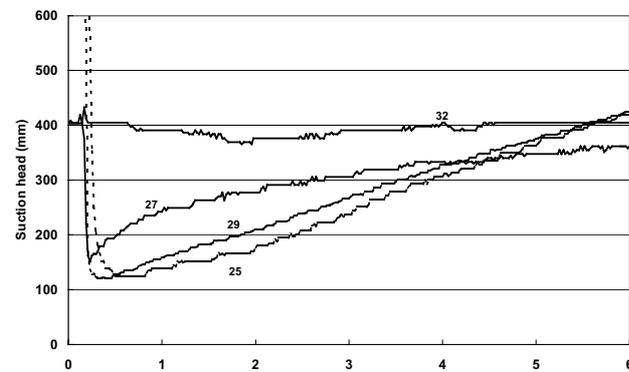
Figure 13. Suction heads in the base of test 3, 13 mm above the GCBD in Test 3.
