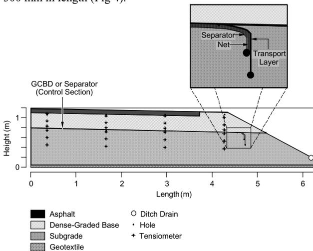
Figure 3. Cross-section of the GCBBD test section showing detail of water collection system for the GCBBD layers.
