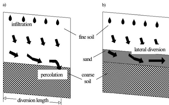
Figure 1. Lateral drainage in unsaturated soil with: a) a capillary barrier and b) a transport layer above a capillary barrier.
