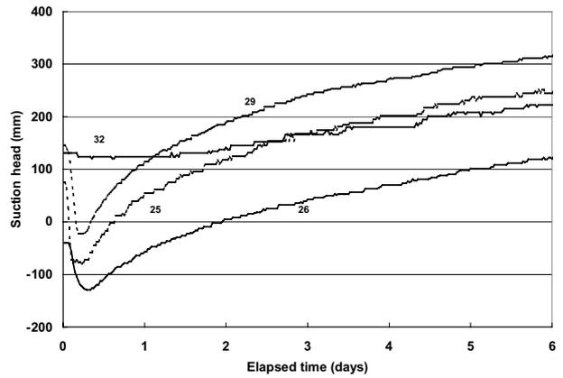
Figure 8. Soil suction heads in the base at 13 mm above GCBD for Test 8.
