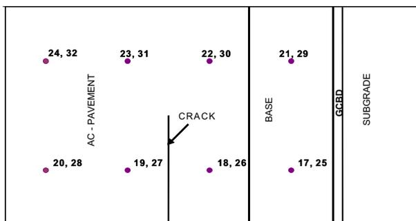
Figure 4. Plan view of test box. The numbers label the tensiometers that are located 25 mm below the base/ subgrade interface (17-24) and 13 mm above the interface (25-32). The box tilts down and to the right.
