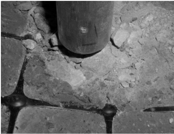
Figure 6. The cone at the test end
