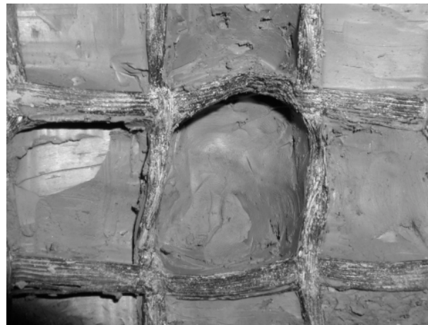
Figure 9. Aperture shape of flexible geogrid after the test
