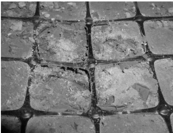
Figure 7. Stiff geogrid after the test
