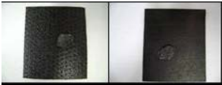
a) High-asperity textured GM b) Low-asperity sand GM Figure 2. Geomembranes used in the tests.
