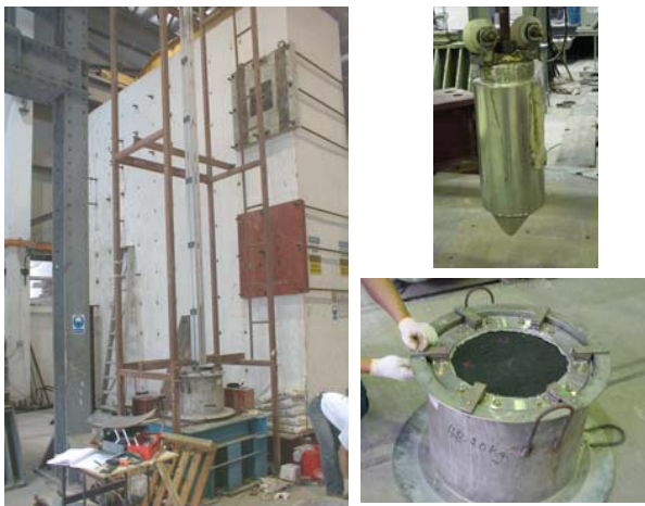
Figure 29. The 5m Impact Rig (left), the impact head (right top), and the metal sand drum with the clamp ring and geotextile sample secured onto it (right bottom).
