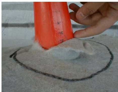
Figure 32. Technique to quantify the damage on the geotextiles - measuring the size of the puncture using cone.
