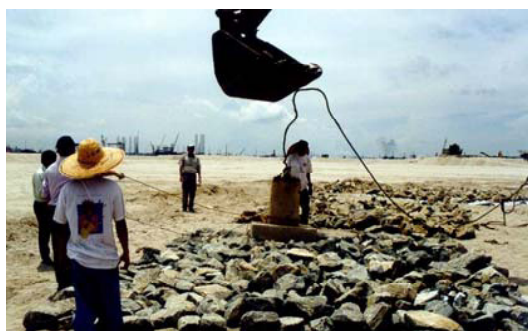
Figure 31. Dropping of standardized stone for Field Drop Test.
