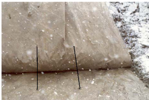
Figure 6. Puncturing of geotextile (SINTEF 1997).
