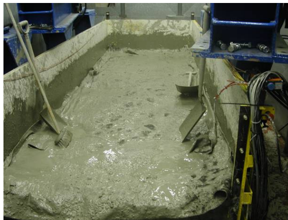
Figure 4. quagmire after use of non-woven separator (as above in figure 3) without membrane or geogrid spacer
