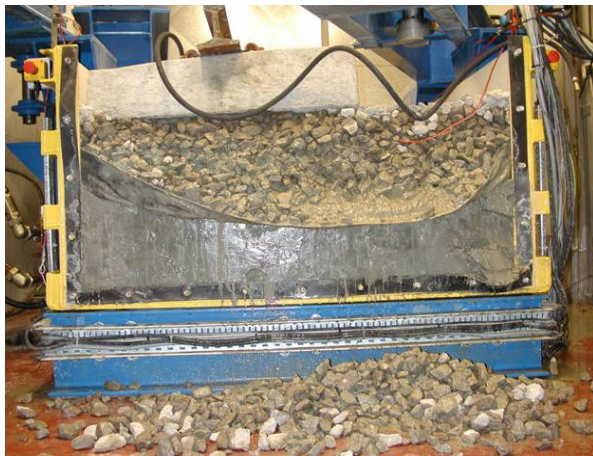
Figure 3. end panel removed noting complete aggregate / sub-soil separation by light-weight non-woven despite high water addition (300-l).
