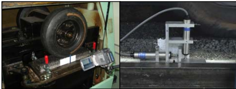
Figure 17. Use of LCPC wheel tracking equipment for reflective crack investigation
