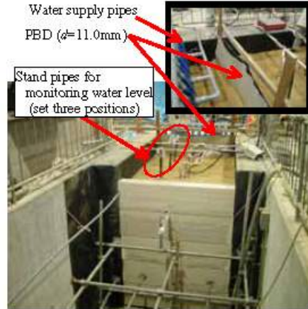
(b) Case2: Embankment with L-shaped geosynthetic drain
