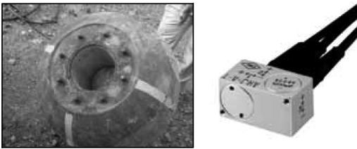
Figure 2. Concrete ball for rockfall and three-dimensional accelerometer.
