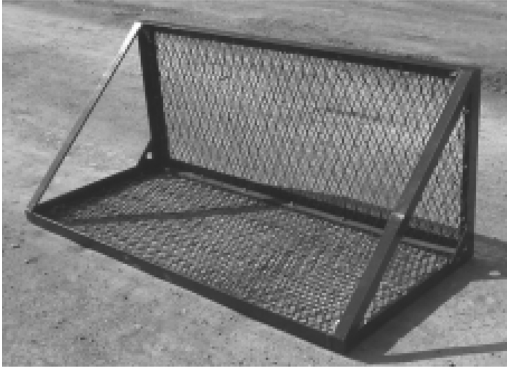
Figure 1. Debris flow trapping fence.
