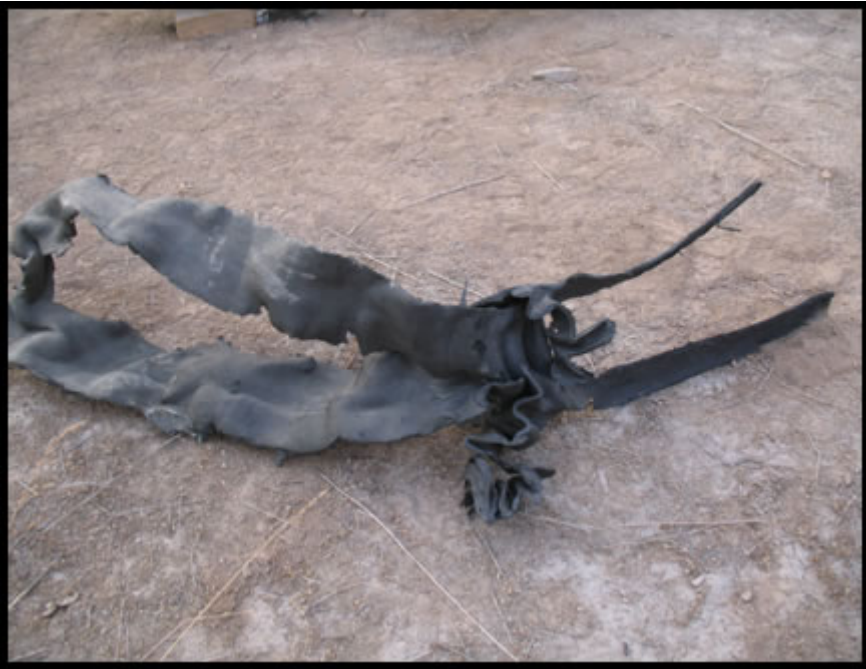
Figure 2. Large piece of broken HDPE liner that caused blockage
