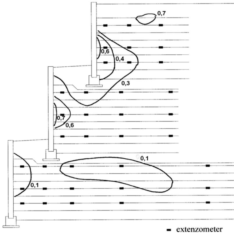
Figure 6. Strain isolines (%) in measuring profile 1
