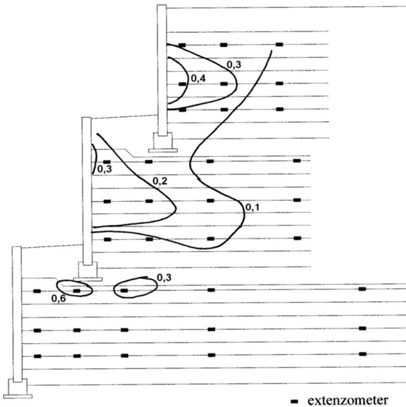
Figure 7. Strain isolines (%) in measuring profile 2
