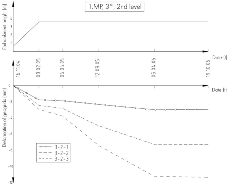
Figure 3. Displacement of the geogrid: MP 1, tier 3, level 2 in time
