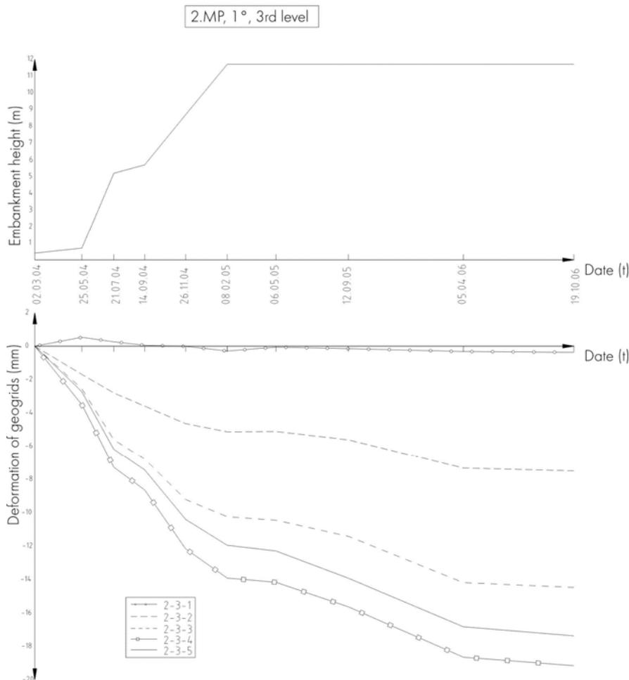
Figure 4. Displacement of the geogrid: MP 2, tier 1, level 3 in time
