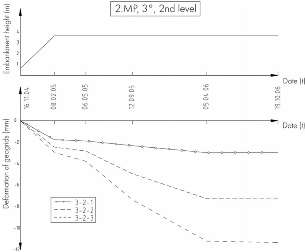
**Figure 5.** Displacement of the geogrid: MP 2, tier 3, level 2 in time
