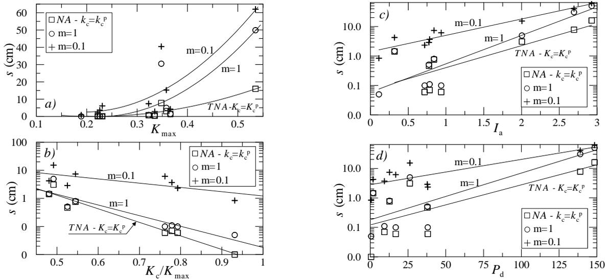
**Figure 5.** Examples of best-fit regression analysis carried out including the strength degradation at the interface. a) relationships between  $s$  and  $K_{\max}$ ; b) relationships between  $s$  and the ratio  $K_c/K_{\max}$ ; c) relationships between  $s$  and  $I_a$ ; d) relationships between  $s$  and  $P_d$ .
