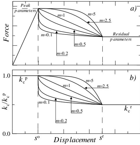
**Figure 1.** a) Scheme of the strain softening force-displacement curves considered in the model by Biondi & Maugeri (2002); b) corresponding yield acceleration degradation paths.
