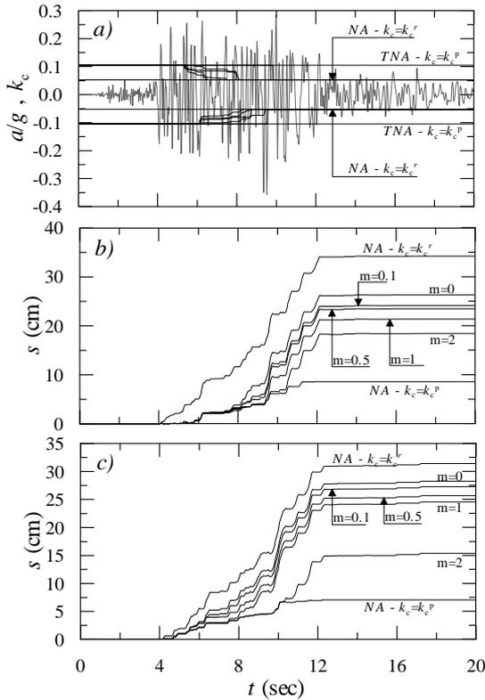
**Figure 2.** Influence of the yield acceleration degradation path on the earthquake-induced permanent displacements. a) yield acceleration degradation path; b,c) permanent displacements computed for the positive and negative side of the accelerogram #E.
