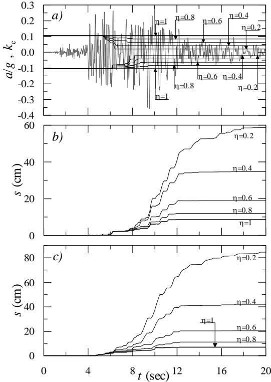
**Figure 4.** Influence of the yield acceleration reduction factor  $\eta$  on the earthquake-induced permanent displacements. a) yield acceleration degradation path; b, c) permanent displacements computed for the positive and negative side of the accelerograms #E.
