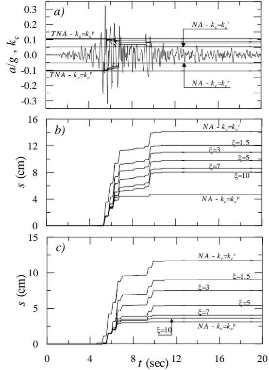
**Figure 3.** Influence of the displacement ratio  $\xi$  on the earthquake-induced permanent displacements. a) yield acceleration degradation path; b,c) permanent displacements computed for the positive and negative side of the accelerogram #H.
