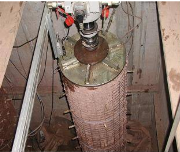
Figure 10. Geogrid coated stone columns (Trunk et.al. 2004)
