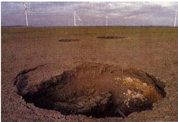
Figure 12. Sinkholes in free field, caused by previous mining, near Wansleben (Germany) (Paul 2004)
