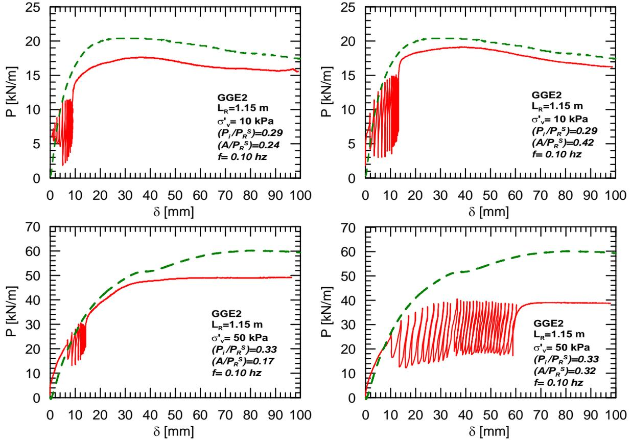
**Figure 3.** Comparison between static and multistage static and cyclic pullout test for geogrid GGE2
