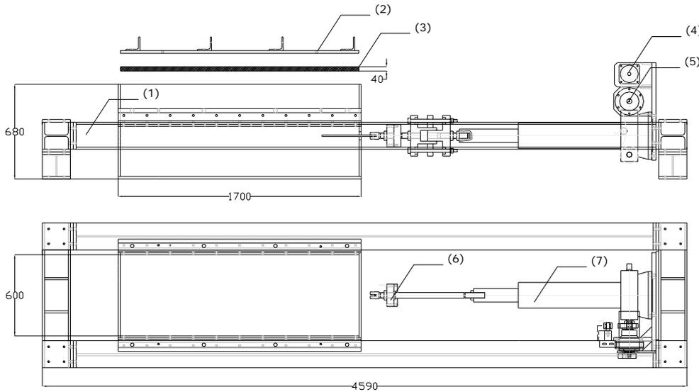
**Figure 1.** Scheme of pullout test apparatus: 1) frame; 2) steel plate; 3) air bag; 4) electric engine; 5) reducer; 6) load cell; 7) electric jack (Moraci and Recalcati, 2006).
