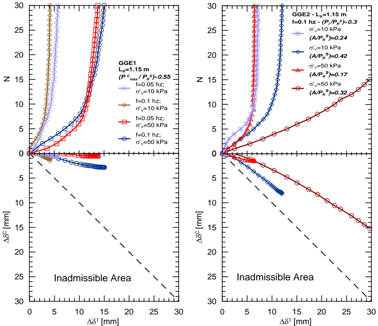
Figure 5. Analysis of pullout behaviour during the cyclic phase: a) geogrid GGE1- b) geogrid GGE2.
