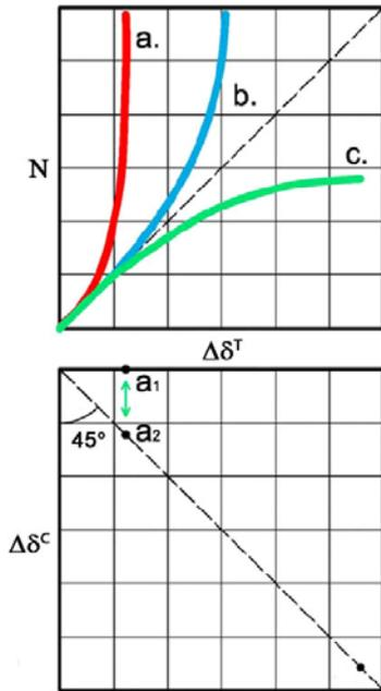
Figure 4. Stability analysis scheme according to Raju and Fannin (1997)
