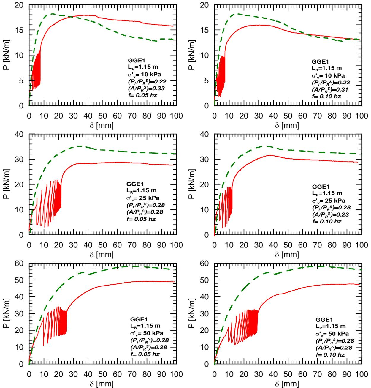
**Figure 2.** Comparison between static and multistage pullout tests for geogrid GGE1
