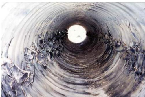
Figure 8 Wall crushing in geopipe
