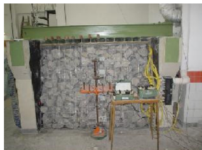
Figure 5: Face of sacks of sand protected by rocks, supported by a metallic grid
