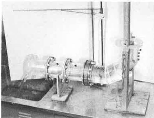
Permeameter with a steady state flow condition.
