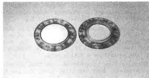
Sample holder with sample inserted into left hand section.
