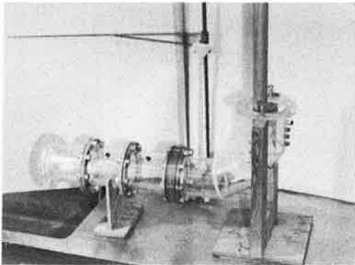
Permeameter positioned over drain and under water inflow pipe.
