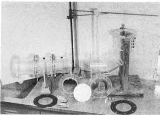
Permeameter with sample holder, gaskets and sample, the white disc.
