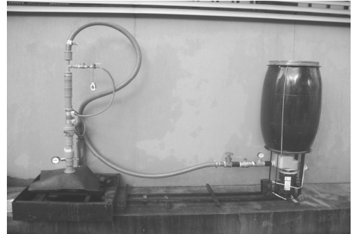
Figure 1 – Equipment for pressurized filling and dewatering.
