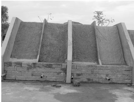
Figure 1. Test cells with and without erosion control geosynthetics.
