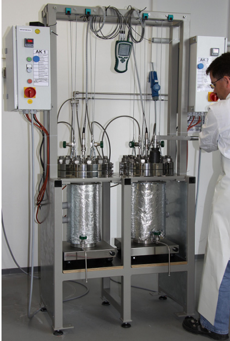
Figure 1. High-pressure autoclave facility in SKZ.
