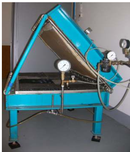
Figure 1. Compressive creep test box
