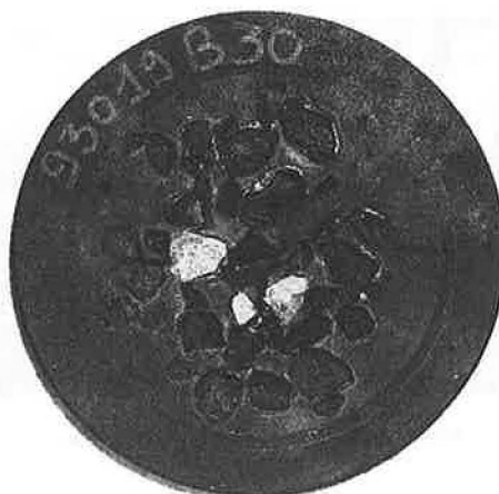
photo 1 10-20mm Aggregate Embedded in Bituminous Geomembrane
