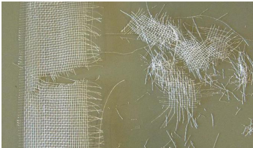
Figure 3. GNT A after 2000 hours of artificial weathering
