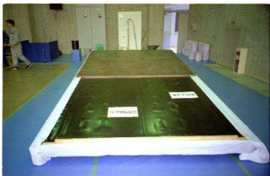
Figure 8. TLS formed by the model test by grouting of intermediate layer
