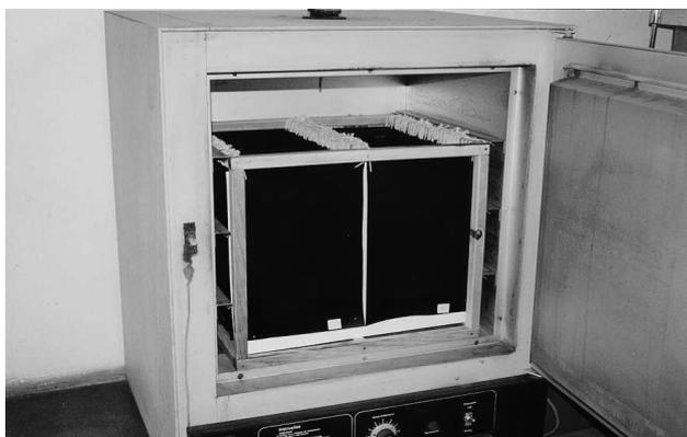
Figure 2. HDPE and PVC geomembranes in the conventional oven
