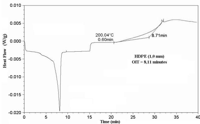
Figure 1. OIT test (HDPE geomembrane – 1,0 mm)
