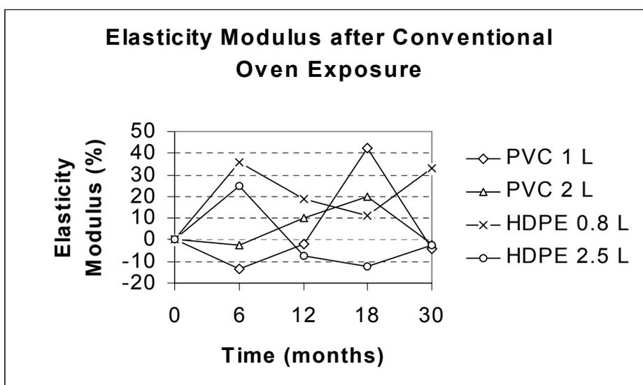
Figure 3. Variation of tensile properties after exposure to heat in a conventional oven
