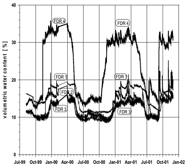
Figure 3. Continuous measurements of volumetric soil water content in the restoration profile between 0.2 m depth (FDR 4) and 0.8 m (FDR 1).
