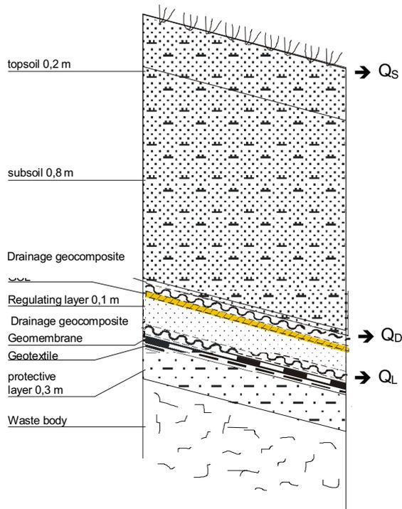
Figure 1. Cross section of the test field.
