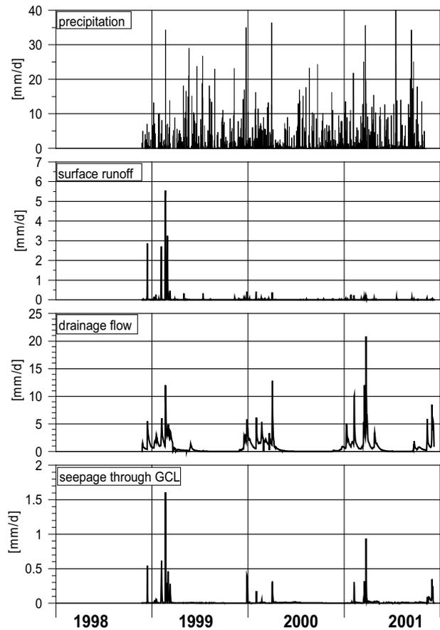
Figure 2. Daily values of precipitation and water flows in the test field
