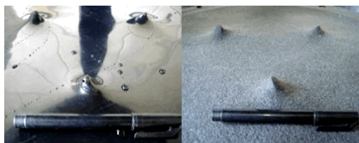
Figure 8. Rupture of HDPE before protective layer failure.
