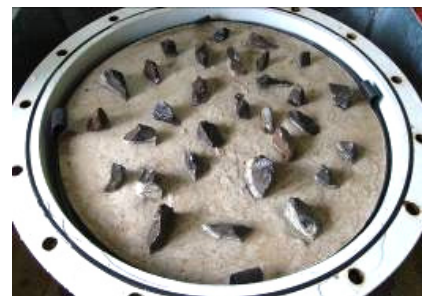
Figure 2. Subangular stones in pressure vessel.
