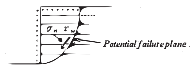
a) shear deformation along potential failure plane
