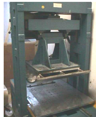
(a) Roller Compactor
