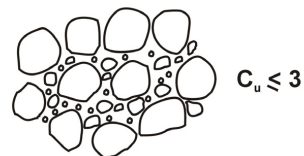
Figure 5. Schematic representation of a soil with a coefficient of uniformity equal to or less than 3.
