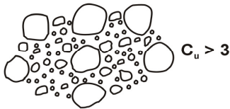
Figure 6. Schematic representation of a soil with a coefficient of uniformity greater than 3.
