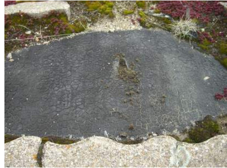
Figure 2. Aspect of the geomembrane surface from site 5 at the time of sampling
