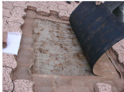
Figure 3. Aspect of the underlying face of the geomembrane from site 6 during sampling
