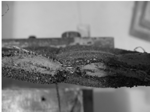
Figure 8. Deformed shape of GCL2 after bentonite expansion.
