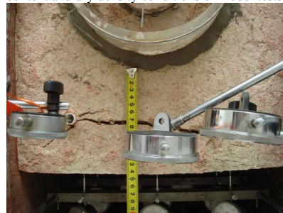
Fig.3 Transverse tension crack occurred after test for No1-1
