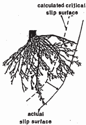
Fig. 6. Schematic diagram of soil reinforced by roots network.
