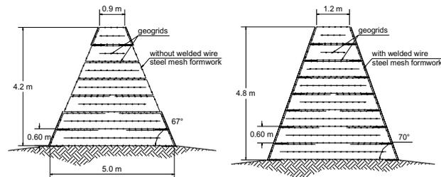
Fig. 2: Sketched cross section of the embankments built for test 4 and 5.
