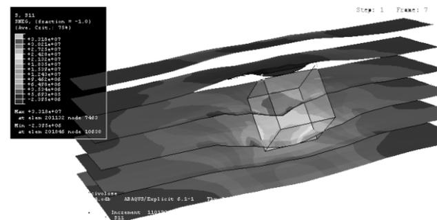
Fig. 7: In-plane stress traction stress distribution on geogrids.
