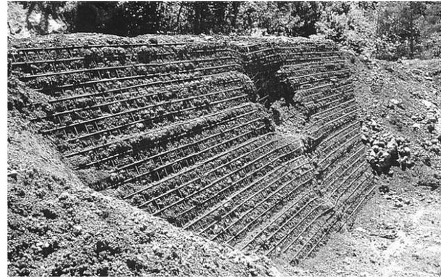
Fig. 3: Front deformation induced by the impact in first test.
