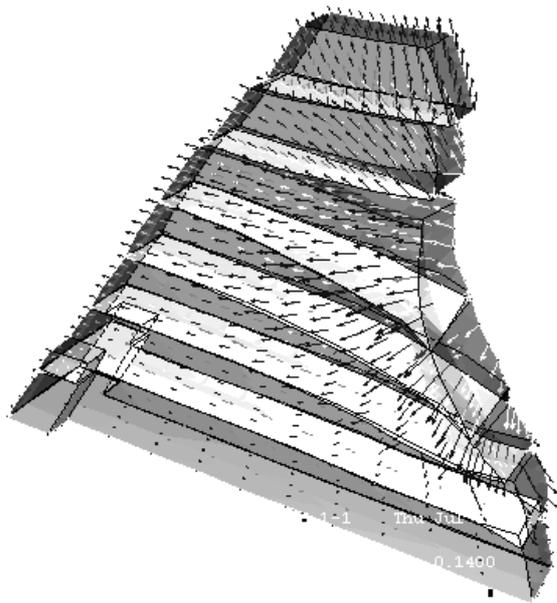
Fig. 8: Displacement vectors in the cross-section after 0.12 s.
