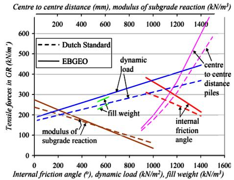
Figure 1. Influence differences safety Dutch and German approach, Lastfall 1 (EBGEO) and RC 2 (Dutch/Eurocode), arching reduction (kappa-model) not included yet.
