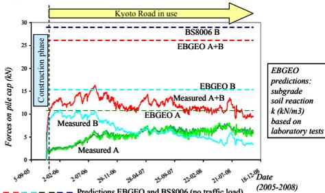
Figure 5. Load distribution in the Kyoto Road, prediction and measurements (Van Eekelen et al, 2010)
