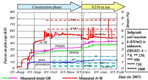
Figure 4. Load distribution in N210, prediction and measurements (Haring et al, 2008)
