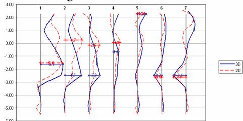
Figure 10. Bending moments in 2D and 3D calculations
