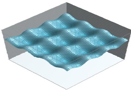
Figure 12. 3D-representation of the surface settlements resulting from Peck (extended to 3D)
