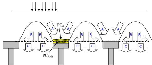
Figure 2. Load distribution in a piled, reinforced embankment
