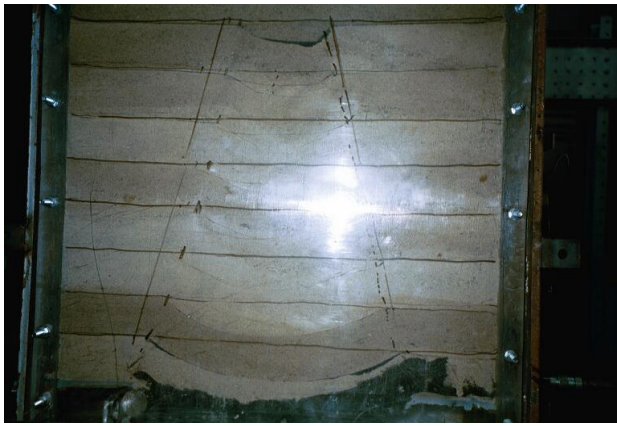
Figure 9. Test No. 4, showing wedge, moisture content 1.3%
