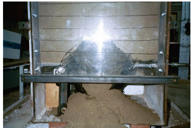
Figure 8. Test No. 3, showing soil arch, moisture content 4.7%.
