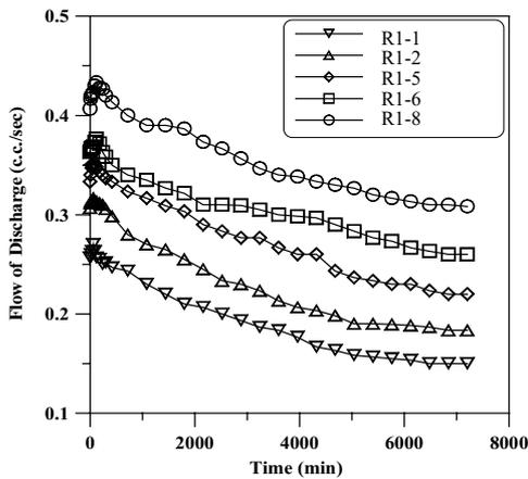
Figure 4. Flow rate of drain layer with geotextile 1
