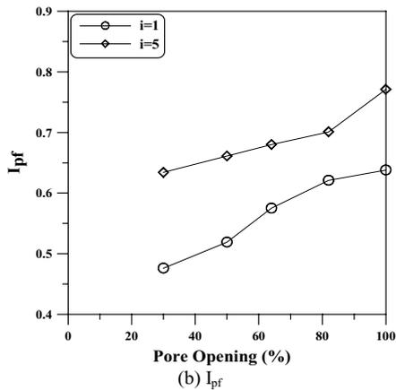
Figure 8. Flow change index vs. opening rate (geotextile 2)
