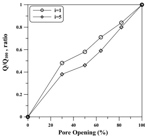
Figure 5. Flow rate vs. opening rate (geotextile 1)
