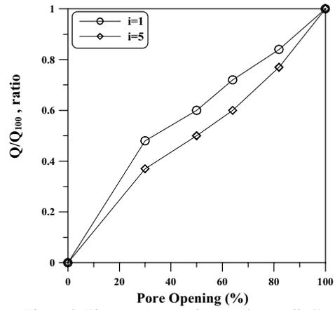
Figure 6. Flow rate vs. opening rate (geotextile 2)
