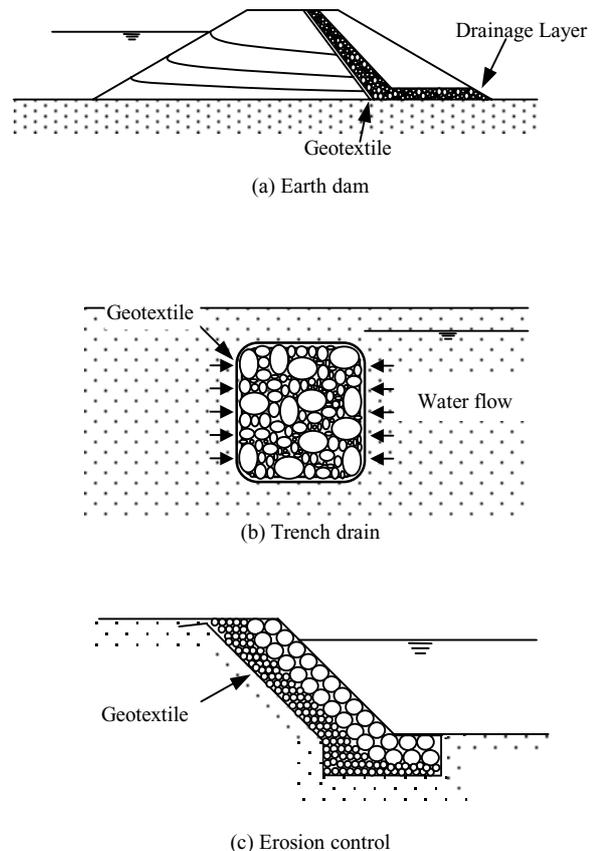
Figure 1. Geotextile in filtration and drainage applications
