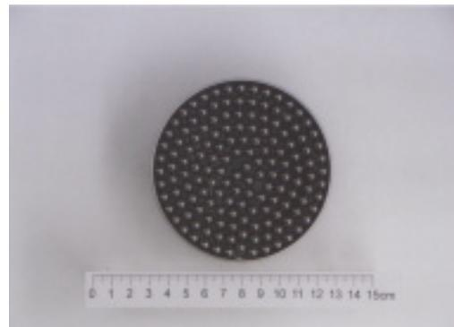
Figure 3. Drain layer of 7-mm steel beads
