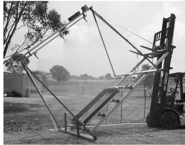
Figure 1 Rainfall simulator, sample tray and frame
