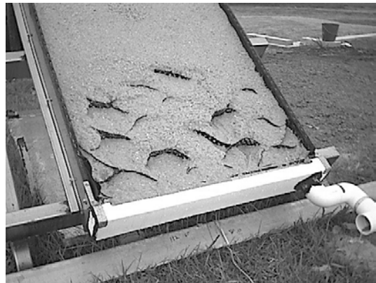
Figure 9 Slumped sand in test bed tray (impermeable base)
