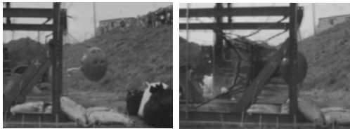
(a) Case 1: without the net (b) Case 2: with the net Photograph 3. Responses obtained from the field tests
