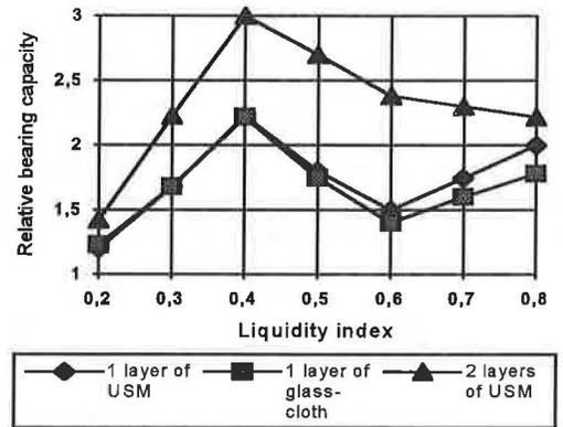
Fig.3 Dependence of the relative carrying capacity of the reinforced foundations constructions on the index of soil flowability.
