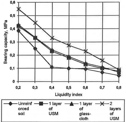
Fig.2 Dependence of the bearing capacity of the reinforced foundation constructions on the liquidity index.
