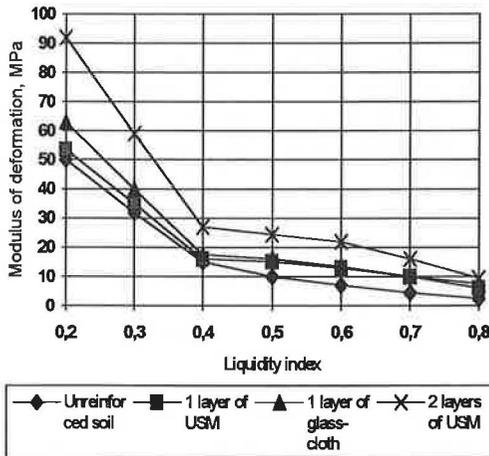
Fig.1 Dependence of modulus of the total deformation of the reinforced foundations constructions on the liquidity index.
