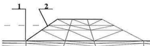
Fig.4 Location of the geomembrane HDPE ( 1 - reinforcing element, 2 - antiferling screen).
