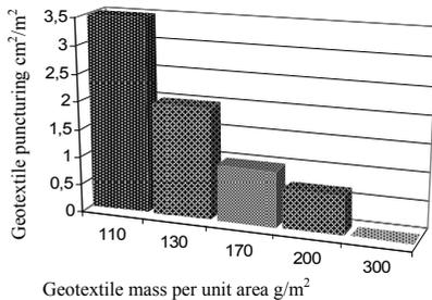
Figure 3. The total area of geotextile punctures cm<sup>2</sup> per m<sup>2</sup> on the second test section
