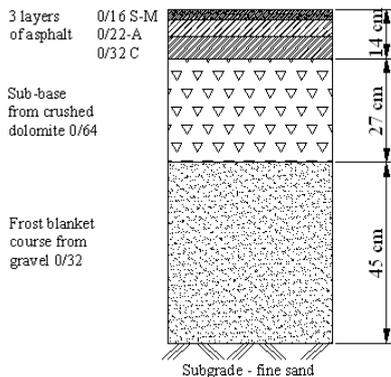
Figure 1. A cross-section of a new road structure
