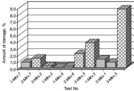
Figure 5. Mean values of geotextiles damage area (GTX1 in lines, GTX2 in mesh)
