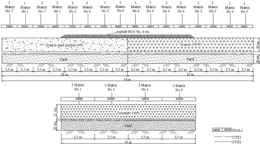
Figure 4. The longitudinal section of the test sections
