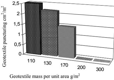
Figure 2. The total area of geotextile punctures cm<sup>2</sup> per m<sup>2</sup> on the first test section
