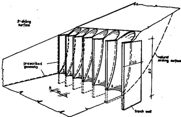
What happens when the soil is removed ? One can imagine with ease the double curved S surfaces as a result of the internal and soil-wall surface frictional resistance and the lateral arching effect. This latter one is well known and called as silo effect in vertical planes. In the given case the lateral earth pressure induces arching effect in the horizontal plane.
