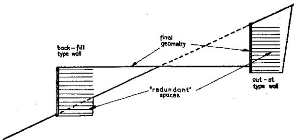
When a backfill-type construction is required, the reinforced earth wall seems to be optimum. But when you have to design a cut-out type retaining wall, there is some redundancy in the reinforced earth type construction, because the technology does not fit to the final geometry (Fig. 1).
