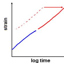
Figure 4: Third step in applying SIM: horizontal shift along log time axis
