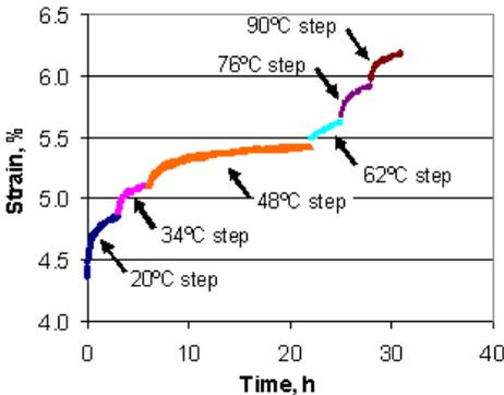
Figure 1. Strain vs Time curve from tensile SIM
