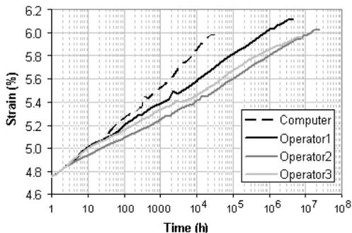
Figure 5: Shifted curves from tensile SIM test at 30% tensile strength
