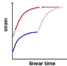
Figure 3: Second step in applying SIM: horizontal shift along linear time axis
