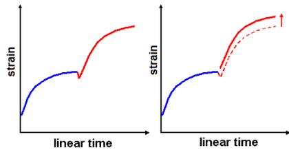
Figure 2: First step in applying SIM: vertical shift
