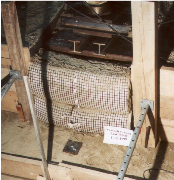
Figure 4. miniature steep slope at loading step \sigma = 850 kPa
